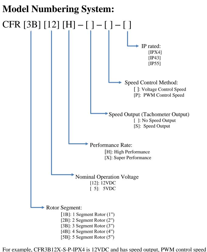
For example, CFR3B12X-S-P-IPX4 is 12VDC and has speed output, PWM control speed and IPX4 rated.
